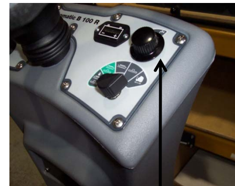
Solution Control Potentiometer
